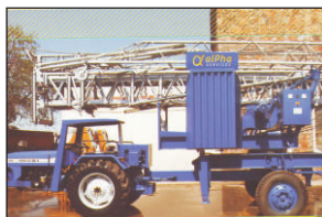
MOBILE TOWER CRANE
